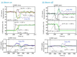
igate the temperature fluctuation caused by the transient heat load change of 17.5 kV and the CMS supply tempeature can be reduced below 0.1 K. The feedforward control should be executed just before the CLI return temperature starts to decrease.
