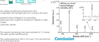
It is expected that the Raman intensities would be able to increase 265-fold at the nominal condition (17 K) because the density of the liquid hydrogen 265 times higher than gaseous hydrogen.
