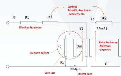
urements/Analyses are accurate for I1, R1, s, f, BH curve
