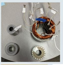
**Engineering evaluation** and deconstruction for design inputs: geometry, resistance, impedance and inductance
