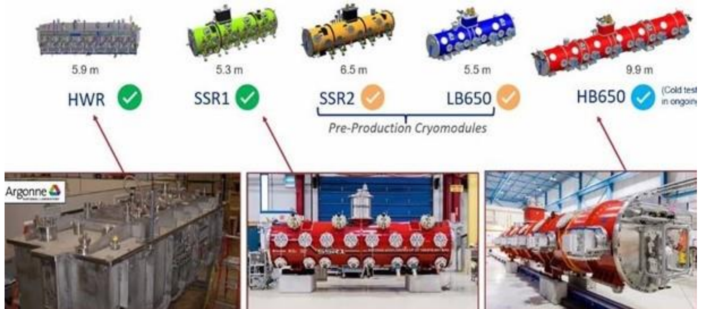
Figure 4. Five types of the PIP2 IT SRF Cryomodules
