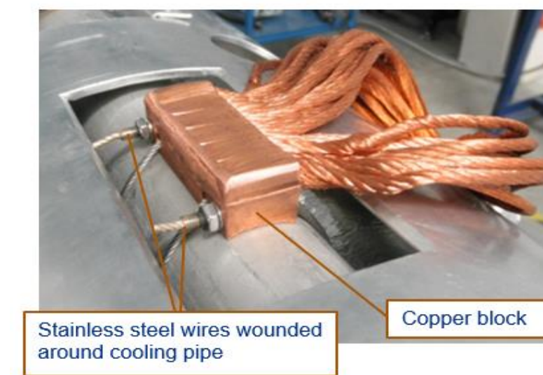
Fig. 1. The simplified example of the operation of an actively cooled thermal shield
