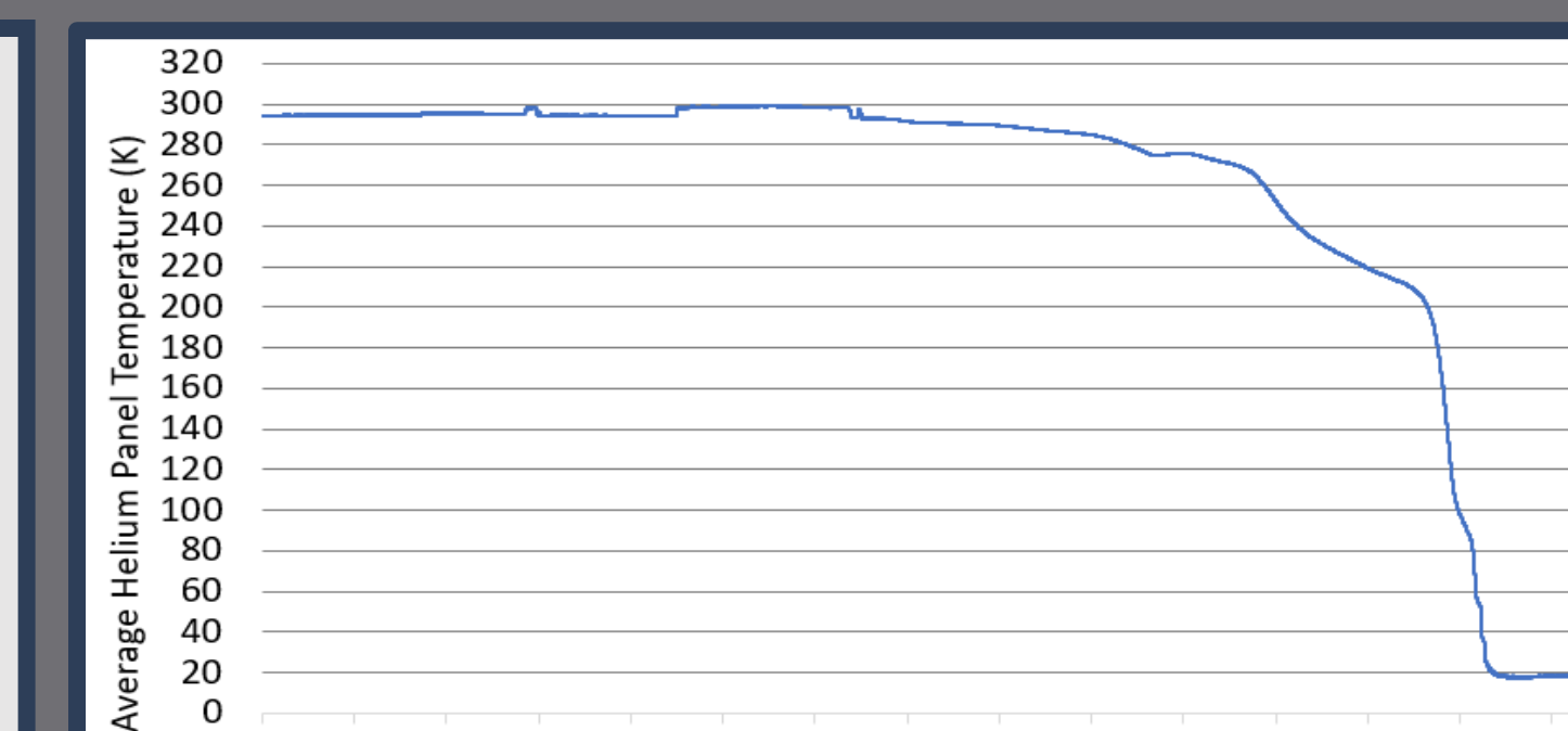
Figure 4: Helium Cryopumping Panel Temperature
