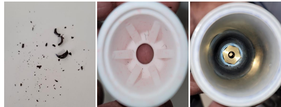
Debris found in Air Filters
