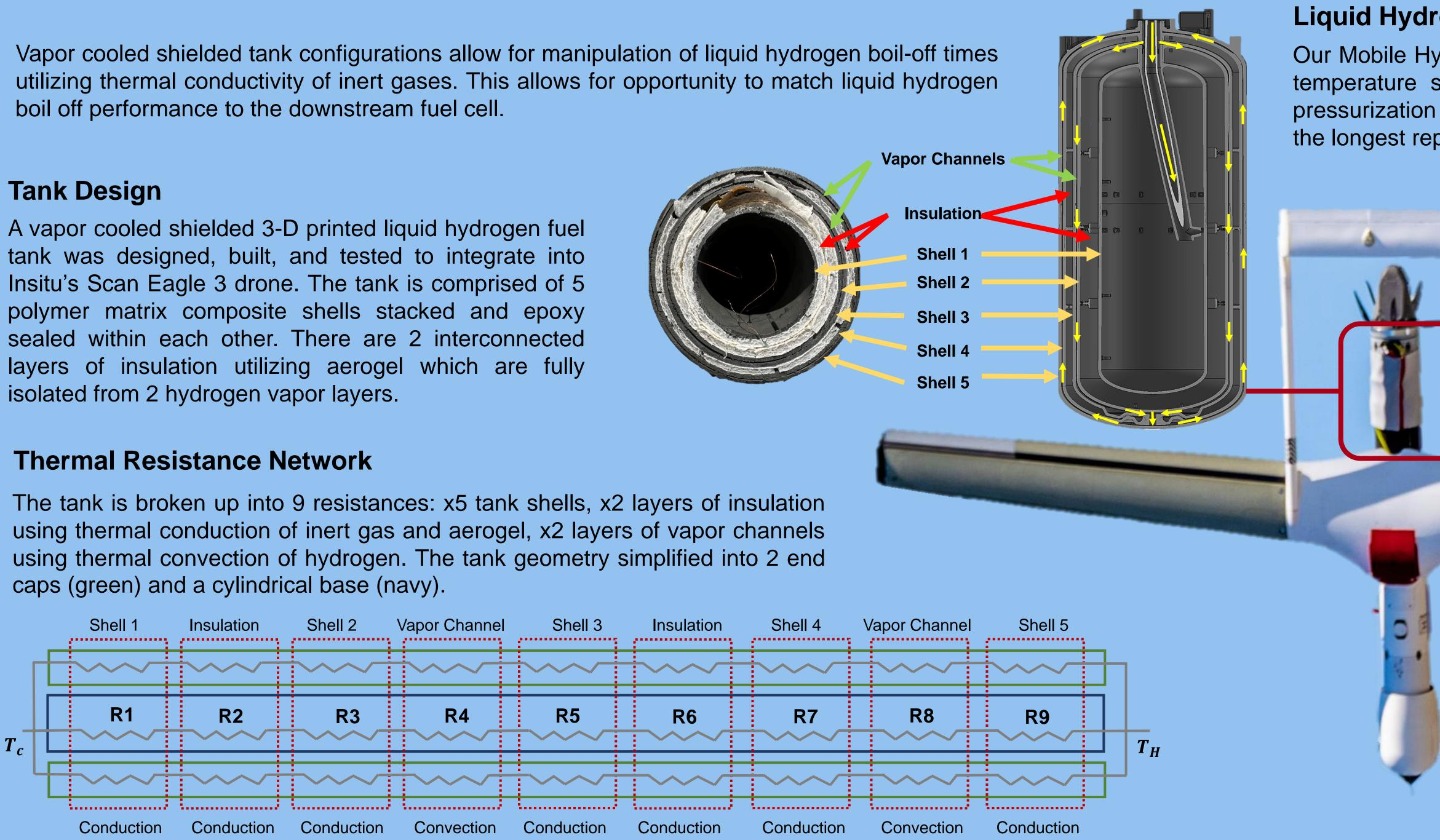
Each individual end cap and cylinder layer is combined in parallel, and each layer is added in series. Energy losses are calculated based off the change in temperature and total resistance. Mass flow rate is calculated based off the energy loss, heat of vaporization, heat capacity and temperature differential. Boil off time is calculated based off mass flow rate and total LH2 mass<sup>1</sup>.
