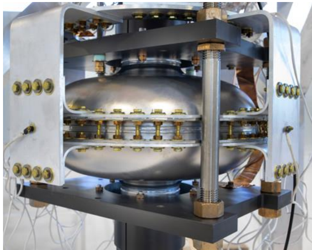
Nb 3 Sn-coated 650 MHz cavity with welded Nb rings for attaching cooling links
