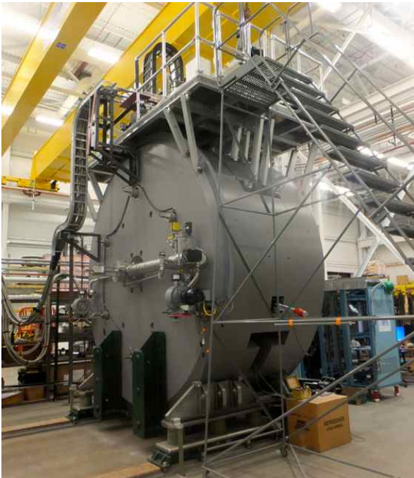
The MSU cyclotron gas-stopper magnet With 167 tons of iron for two poles. Each pole has a cryostat with 3 coolers. Total cold mass is 2.3 tons.
