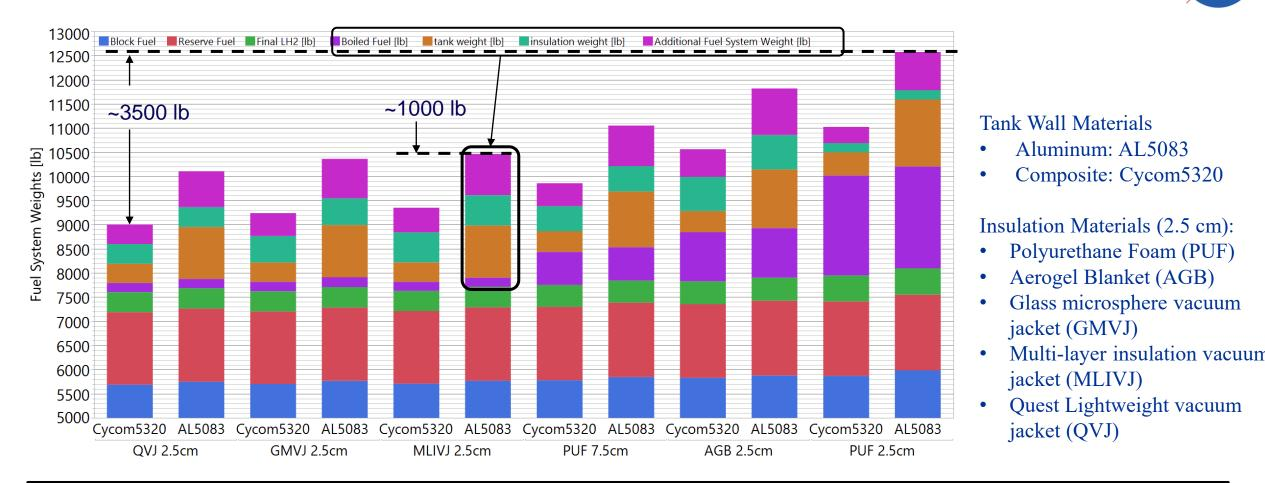
Polyurethane foam is light (lower fuel system mass), but the higher boiloff requires additional fuel to be carried. Which results in larger tanks, increased aircraft structural weight, and worse fuel burn
