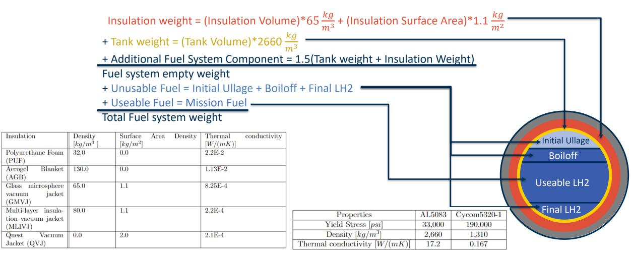
Tank weight buildup is important to assess impacts of weight on aircraft fuel burn
