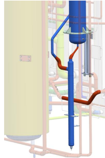
Figure 8: 3D model showing configuration after installation of heaters
