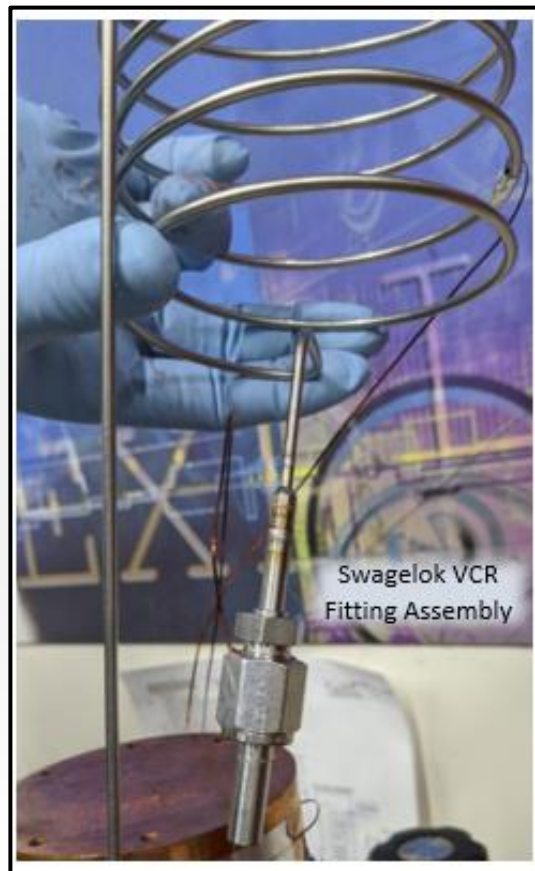
Test fitting assembly prior to TVAC installation
