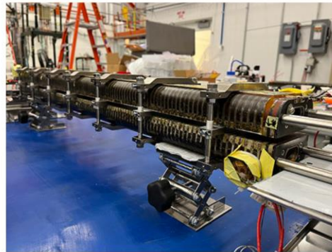
The Nb 3 Sn undulator is the product of a long-running collaboration between Argonne, Lawrence Berkeley National Laboratory, and Fermi National Accelerator Laboratory (photo by Argonne National Laboratory).
