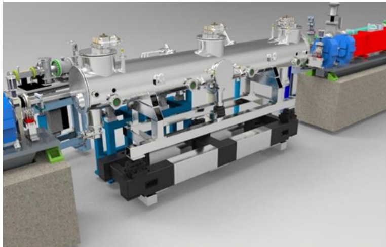
3D sketch of APS-U ID straight section with SCU installation
