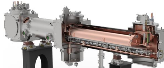
4.8-meter long SCU cryostat, 20" diameter vacuum vessel
