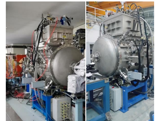
SCU installed in SSRF storage ring
