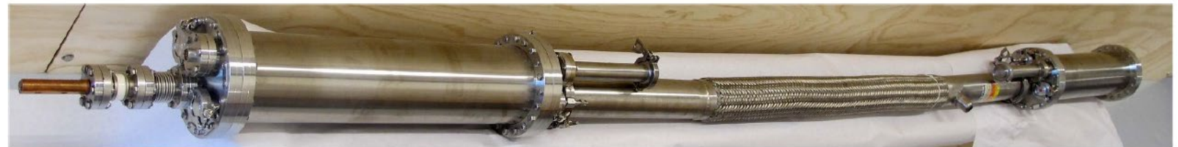
van der Laan "A turnkey gaseous helium-cooled superconducting CORC® dc power cable with integrated current leads" (2022)
