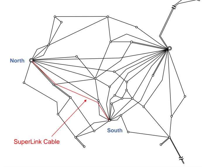
A major challenge nowdays of the 110 kV network in Munich is the off-peak times within the city, when the power generated at the southern substation should not only be available for Munich, but exported to external networks (South to North).
