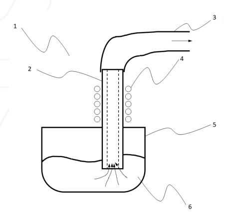
Filling Cu pipe with molten Li under Ar atmosphere. <u>Problem:</u> Dissolves Cu into Li, increases resistivity. <u>Potential solution:</u> Shrink and insert Li rod into Cu pipe.
