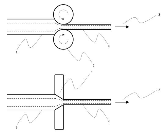
Drawing wire from cylinder assembly. <u>Problem:</u> Work hardening of Cu requires periodic annealing, melting Li, dissolving Cu into Li. Solution: ??
