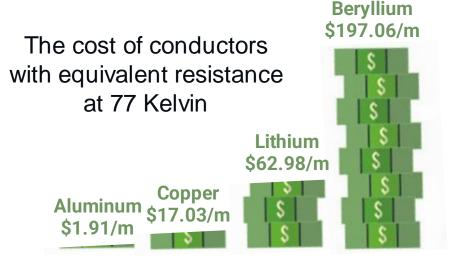
Lithium's intrinsic thermal control enables the selection of conductor size by the optimal trade-off between wire mass and resistive energy loss instead of by the maximum permissible wire temperature. Leading to smaller, lighter, and cheaper conductors.
