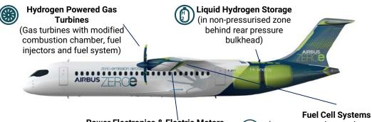
Power Electronics & Electric Motors (powered by the fuel cells and injecting energy onto the turbofan shaft )
