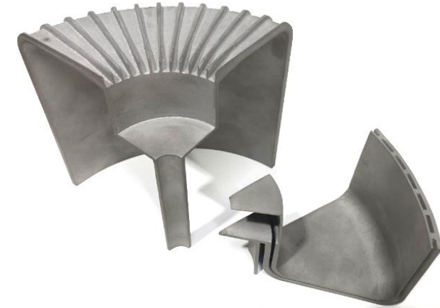
Sectioned components of AM stainless steel superconducting rotor cooling core
