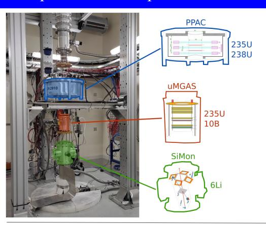
The setup to measure the neutron flux consisted of solid state detectors (SiMon) and gas detectors (uMGAS, PPAC), employing (n, charged-particles) and (n,f) reactions on samples considered as standard.
