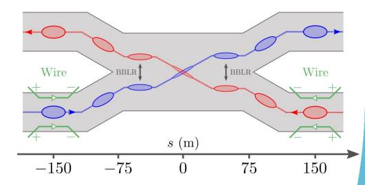
"If the optics and layout conditions ( $\beta$ -aspect ratios, wire distance, etc.) **cannot be met**, wire currents and distances should be used for **cancelling the LR leading order effect**, i.e. **octupole-like tune-spread**."
