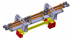
1 assembly/side/IP  $\rightarrow$  1 assembly = 3  $\times$  1-m wire modules/beam 1 module can carry 150 A  $\rightarrow$  450 Am per beam/side/IP
