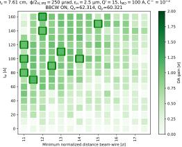
HL-LHC v1.5, no MS.10,  $N_b=1.8 \times 10^{11}$  ppb,  $\beta^*_{IP1/5}=30$  cm,  $\phi/2_{IP1/5}=190$  µrad  $\sigma_z = 7.61 \text{ cm}, \ \varphi/2_{H, IP8} = 250 \ \mu rad, \\ \epsilon_n = 2.5 \ \mu m, \\ Q' = 15, \\ I_{MO} = 100 \ A, \\ C^- = 10^{-3}$
