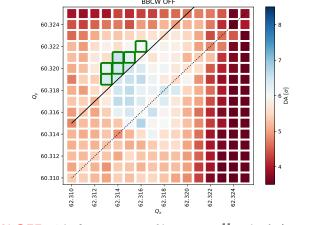
$\begin{array}{l} HL\text{-LHC v1.5, no MS.10, } N_b \!=\! 1.8 \times 10^{11} \text{ ppb, } \beta^{*}_{|P1/5} \!=\! 30 \text{ cm, } \varphi/2_{|P1/5} \!=\! 225 \text{ µrad} \\ \sigma_z \!=\! 7.61 \text{ cm, } \varphi/2_{H, |P8} \!=\! 250 \text{ µrad, } \epsilon_n \!=\! 2.5 \text{ µm, } Q' \!=\! 15, I_{MO} \!=\! 100 \text{ A, C}^{-1} \!=\! 10^{-3} \text{ BGW OFF} \end{array}$
