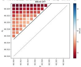
$\begin{array}{l} \text{HL-LHC v1.5, no MS.10, N_b=1.8 \times 10^{11} \text{ ppb, } \beta_{\text{IP1/5}}^{}=30 \text{ cm, } \varphi/2_{\text{IP1/5}}=190 \text{ } \mu\text{rad}} \\ \sigma_z=7.61 \text{ cm, } \varphi/2_{\text{H,IP8}}=250 \text{ } \mu\text{rad}, \\ \epsilon_n=2.5 \text{ } \mu\text{m, } Q'=15, \\ \text{I}_{MO}=100 \text{ } \text{A}, \\ \text{C}^-=10^{-3} \text{ } \text{B}_{\text{CW}} \text{ } \text{OF} \end{array}$
