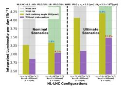
Performance gain by extending the levelling reach/time:  $\rightarrow$  w/ CC, BBCWs push  $\int \mathcal{L}dt$  by 1.8-3.4%  $\rightarrow$  w/o CC, BBCWs push  $\int \mathcal{L}dt$  by 6.2-12.6%
