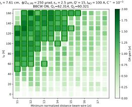
HL-LHC v1.5, no MS.10,  $N_b=1.8 \times 10^{11}$  ppb,  $\beta^*_{IP1/5}=30$  cm,  $\phi/2_{IP1/5}=190$  µrad  $\sigma_z$  = 7.61 cm,  $\phi/2_{H,\,IP8}$  = 250 µrad,  $\epsilon_n$  = 2.5 µm, Q' = 15,  $I_{MO}$  = 100 A,  $C^-$  = 10^{-3} BBCW ON,  $Q_x$  =62.314,  $Q_y$  =60.321
