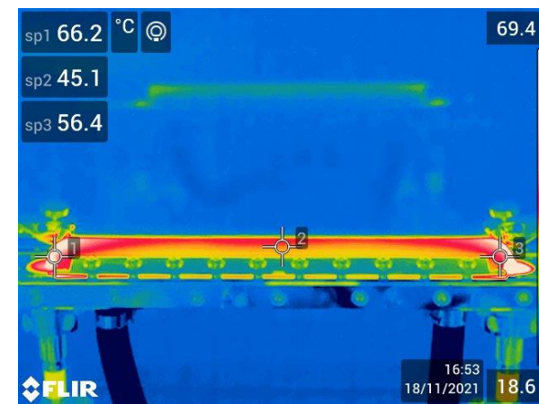
150 A; 1-mm wire; 1 Nm on all screws
