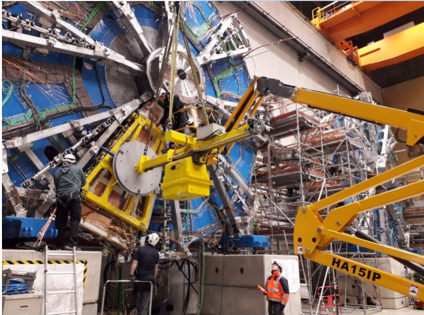
Installing the sector
