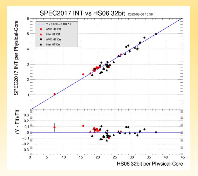
SPEC2017 intrate vs HEPSPEC06-32bit (per physical core)
