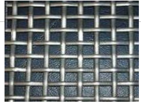
Wire thickness (25 \mu m) = 1/4 human hair 10 wires per mm
