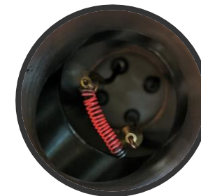
W filament, 10 -2 mbar H 2
