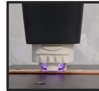
Atmospheric pressure plasma, 1 bar H 2 +N 2
