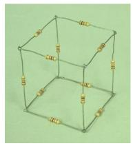
Write a program to solve for the currents in a resistor cube. There are 12 resistors, one along each edge. A voltage source is connected across a body diagonal of the cube.
