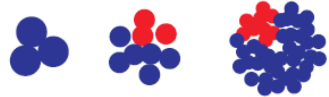
Cable cross section from JackPot simulation
