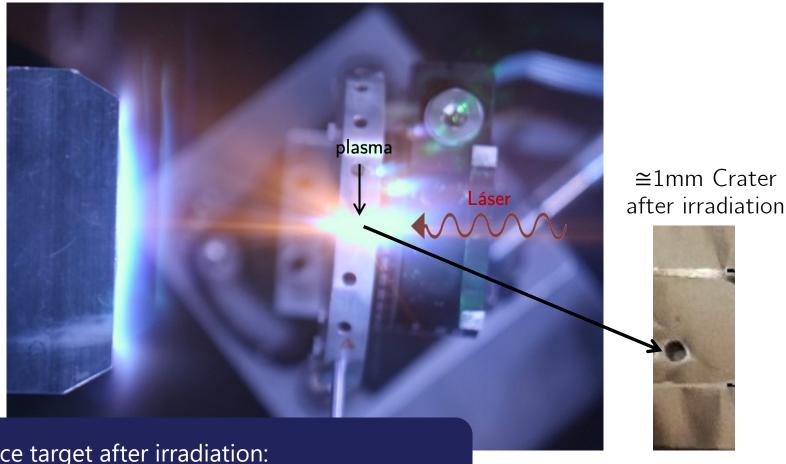
⇒ Replace target after irradiation: micron precision alignment required!
