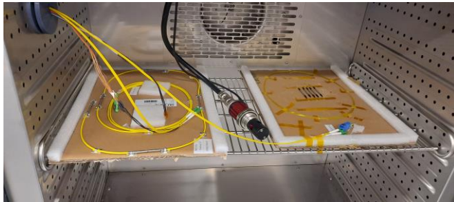
RH + T Fiber Optic Sensors testing (100 PVs)
