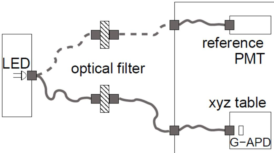
Fig.1 General scheme of PDE measurement
