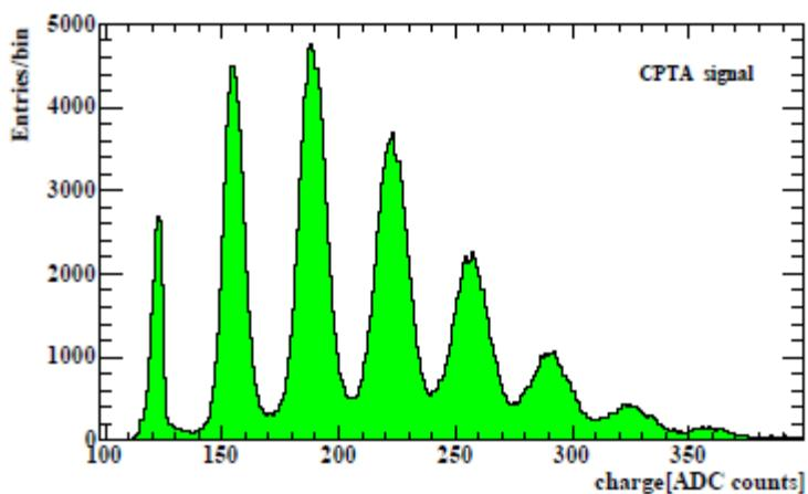
Signal spectra obtained with CPTA detector by short, low intensity LED at  $\lambda = 600 \pm 3\text{nm}$ . Each peak corresponds to a number of detected photons.
