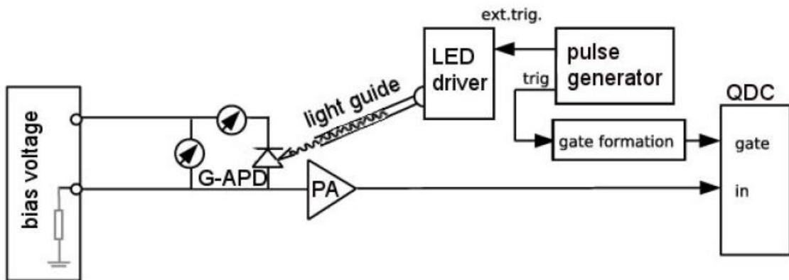
Fig.2 Schematic SIPM readout
