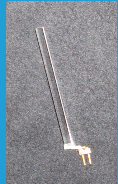
Assembly of LYSO and MPPC, thanks to A.Rudge, P.Weilhammer
