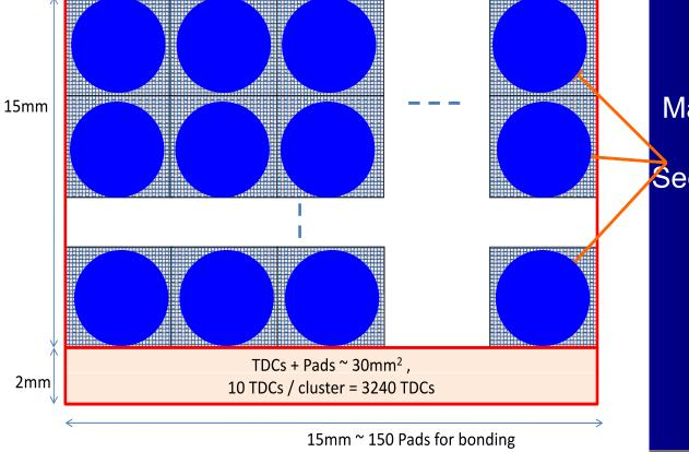
Matrix of 18x18=324 fibers **Φ**≤ 780μm L=10mm Section.cylindrical or square LYSO:Ce, LuAG:Pr,...
