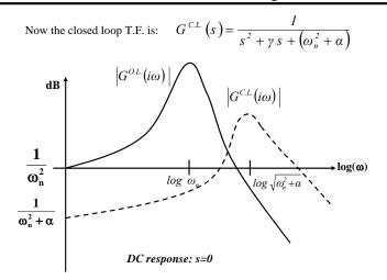
So the effect of the proportional feedback in this case is *to increase the bandwidth of the system* (and reduce gain slightly, but this can easily be compensated by adding a constant gain in front...)
