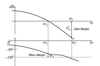
The closed loop is stable if the phase of the unity crossover frequency of the OPEN LOOP Is larger than-180 degrees.
