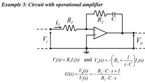
It is convenient to derive a transfer function for a circuit with a single operational amplifier that contains input and feedback impedance:
