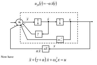
So effect off differential feedback is to increase damping
