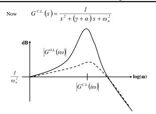
So the effect of differential feedback here is to "flatten the resonance" i.e. damping is increased.
