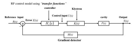
A transfer function of a <u>linear</u> system is defined as the ratio of the Laplace transform of the output and the Laplace transform of the input with I. C .'s =zero.
