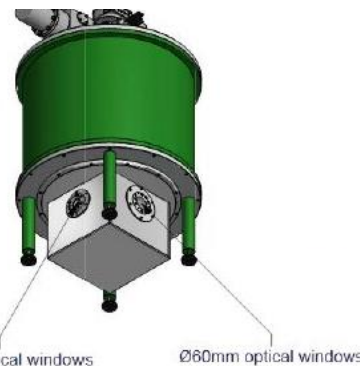
split pair cryogen-free magnet system for combined magneto-optical and FMR measurements
