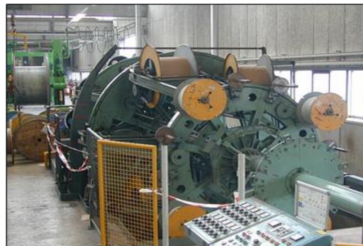
Planetary assembling machine for the final conductor
