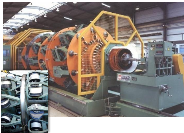
Planetary cabling machine for the petal
