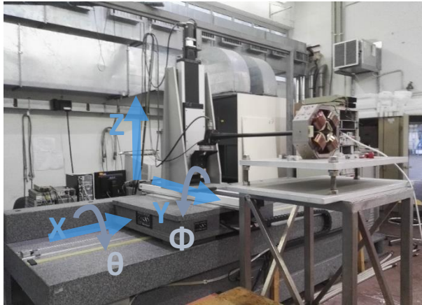
5-axes digital Movement device equipped with Hall Probe
