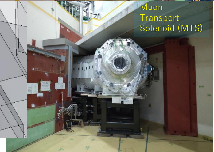
Transport solenoid is installed and cold tested
