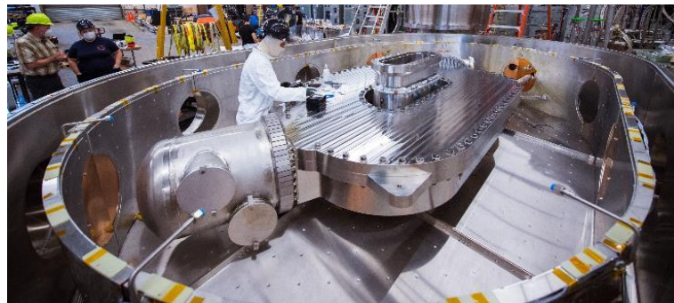
The SPARC Toroidal Field Model Coil (large-scale 20 T 110 MJ coil)
