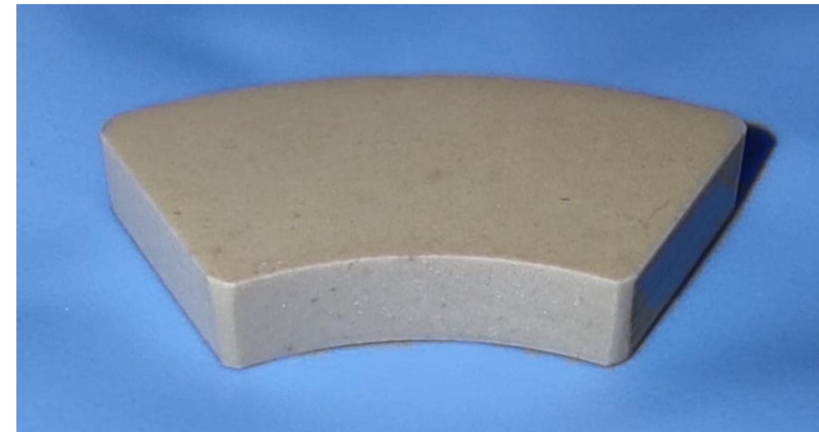
Sample Ceramic: Optical polish surface finish surface area of 75 mm 2 to set capacitance
