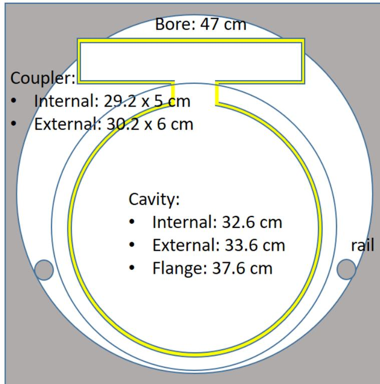
Radial waveguide may not fit within the 47 cm bore
