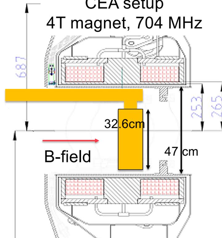
47 cm bore of the MICE AFC magnet will tightly fit the cavity
