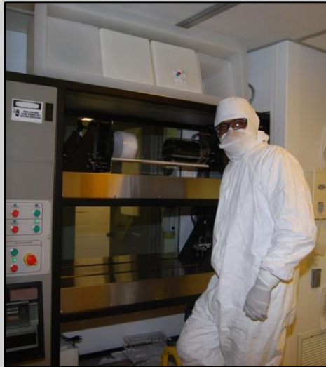
Furnaces for dry oxidations and annealings
