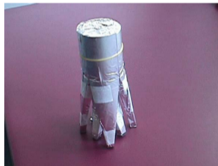
Fig. 13. A photograph of the regular PIBETA active target. Acrylic tapered light guides are glued to nine optically isolated target segments.
