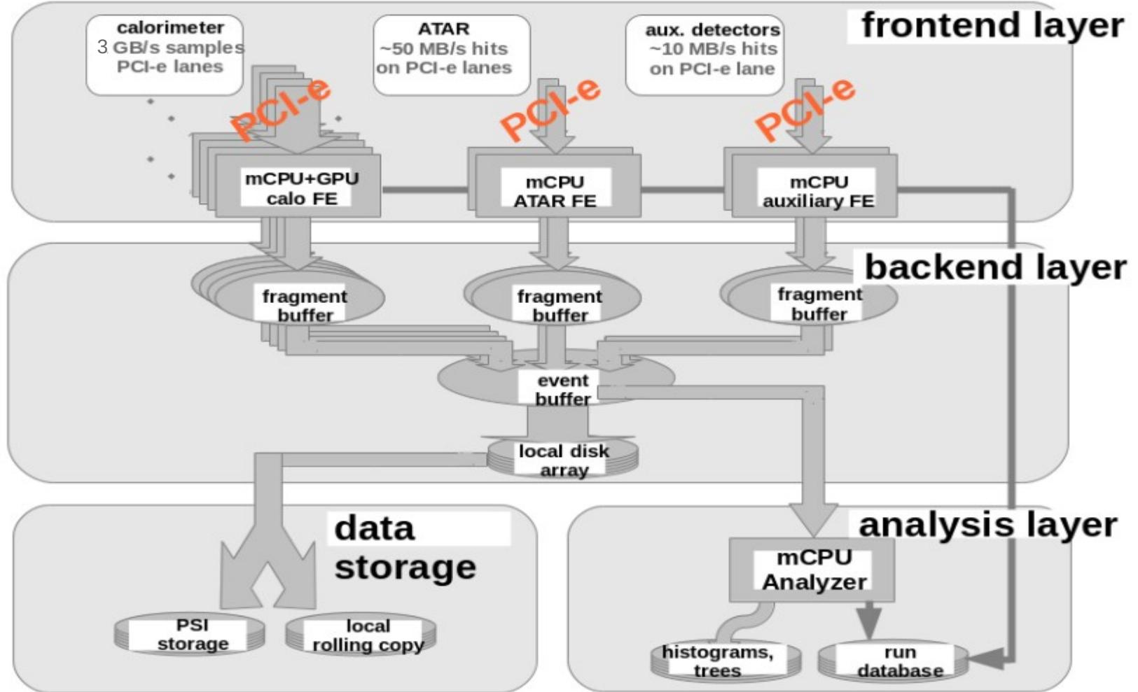
Schematic showing frontend layer for data readout / compression, backend layer for event assembly / data storage, and the analysis layer for online monitoring
