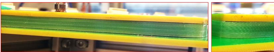
GAPS AT THE INTERFACE BETWEEN THE EXTERNAL FRAME AND PCBs
