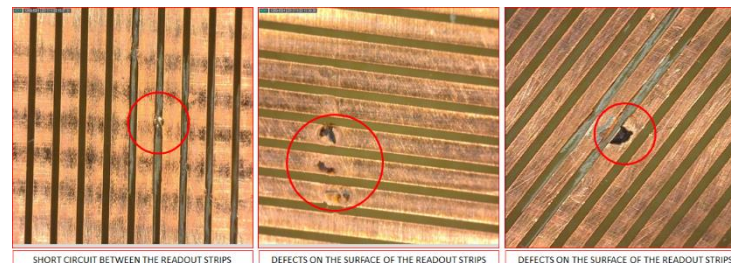
Microscopy photos of the readout strips showing some examples of defects and short circuits between the readout strips.
