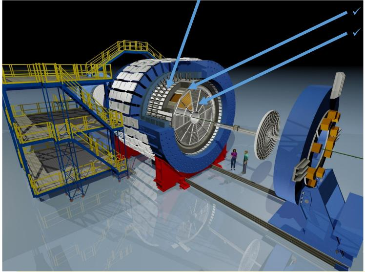
TOF: Time of flight, particle identification TPC: Tracking, momentum and dE/dx
