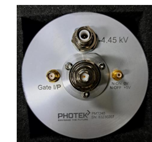
Fig.12 PMT: PHOTEK PMT240 (60 ps rising time)
