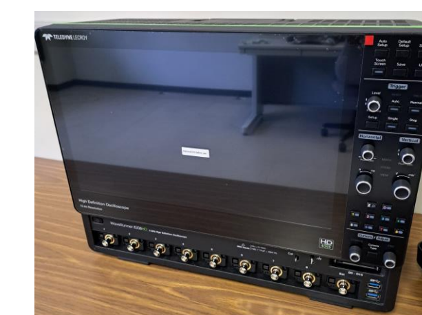
Fig.10 Oscilloscope: WaveRunner 8208HD (10GS/s, 8ch)
