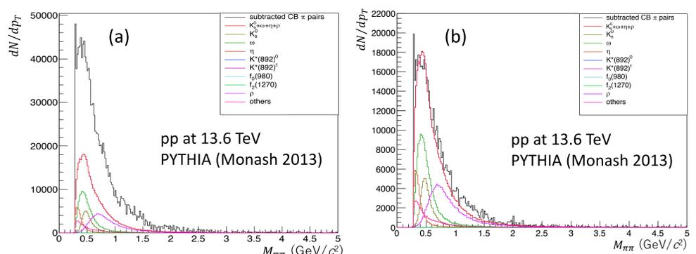
Fig. 5 Comparison between pion pairs cocktail and mass spectrum after subtraction of uncorrelated BG (a) including ambiguous tracks, (b) no ambiguous tracks
