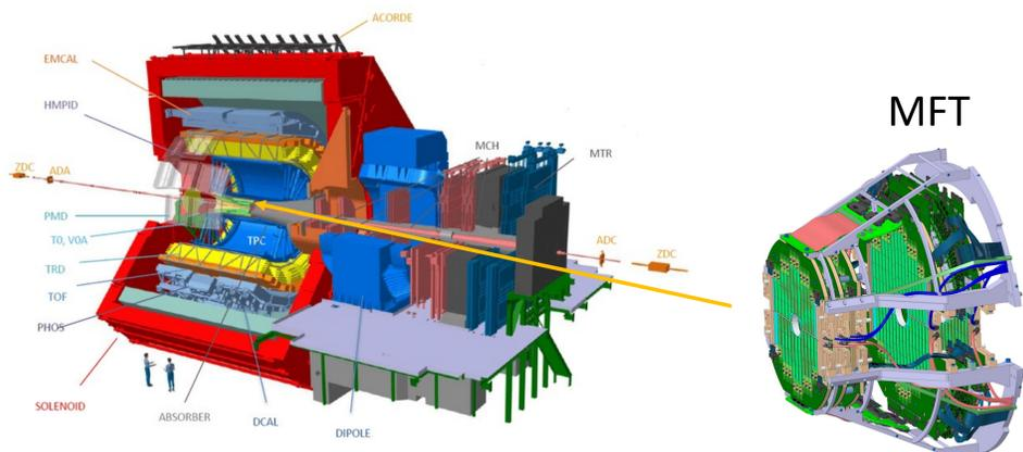
Fig. 3 ALICE detector and Muon Forward Tracker
