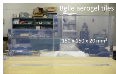
Figure 6: Belle aerogel tiles (left) and aerogel transmission function (right).
