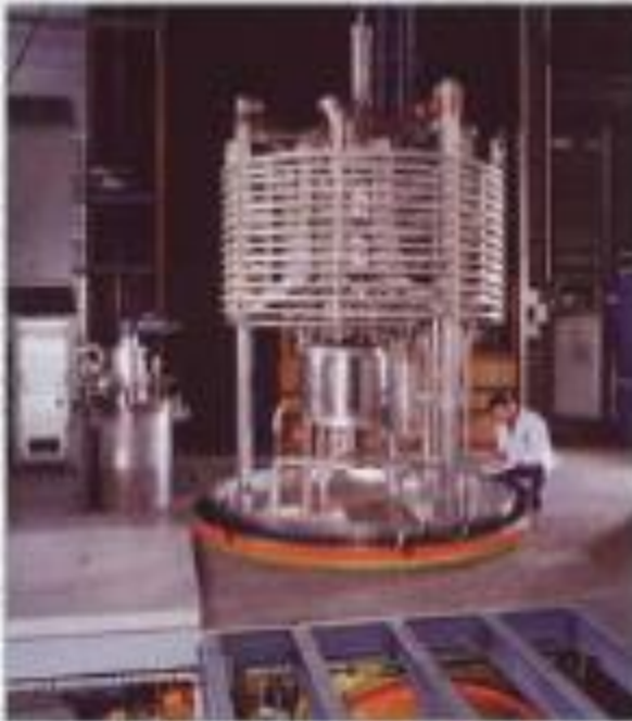
Helium vessel 40 mm diameter, 10 m long, 1.25 MPa.
